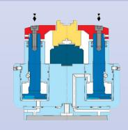
Two long stroke jaws compact self-centering device
