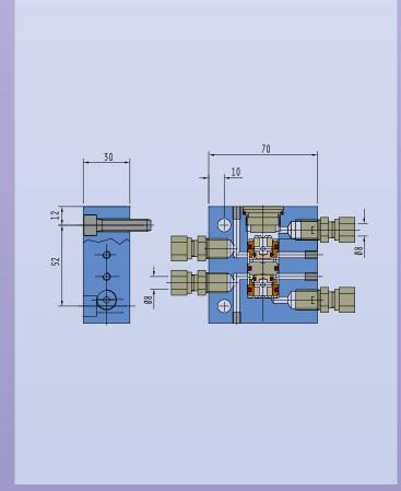
• Rotating distributing groups for every kind of pneumatic cylinder without bar passage, with stroke control option
